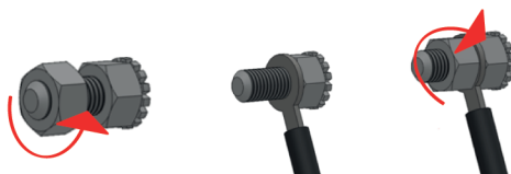
Figure 3. Connecting the unit to an electrical equalizing system
